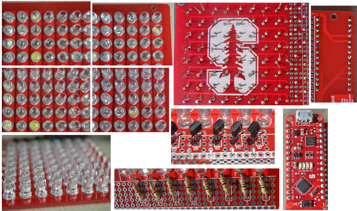
Figure B.17: Pictures for LED display debugging activity. Students could ask to inspect various parts of the circuit board to try and find where the problem was. Upper and lower left: inspection of the LEDs, Upper right: two pictures show back of PCB board, Middle: inspection of transistors, Bottom middle: inspection of resistors, and Bottom right: inspection of Arduino. In the upper right picture showing the back of the circuit board where the Arduino socket connects to the board, you will find the 6th pin down on the left is missing solder.
