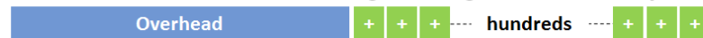
Figure 3.1: Comparison of functional unit energy with that of a typical RISC instruction in 90nm. Strategy for amortizing processor overheads includes executing hundreds of low-power operations per instruction.
