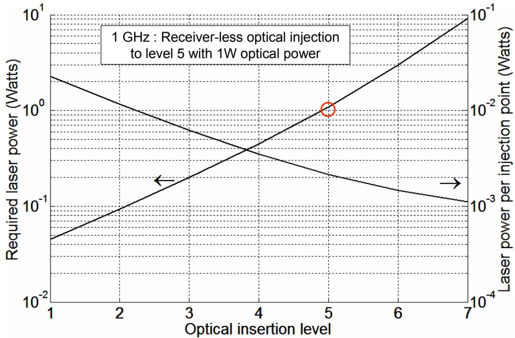
Figure 3.6 Laser output power required for optical clock injection vs. insertion level. (Right) Laser power required per injection point (1 GHz)
