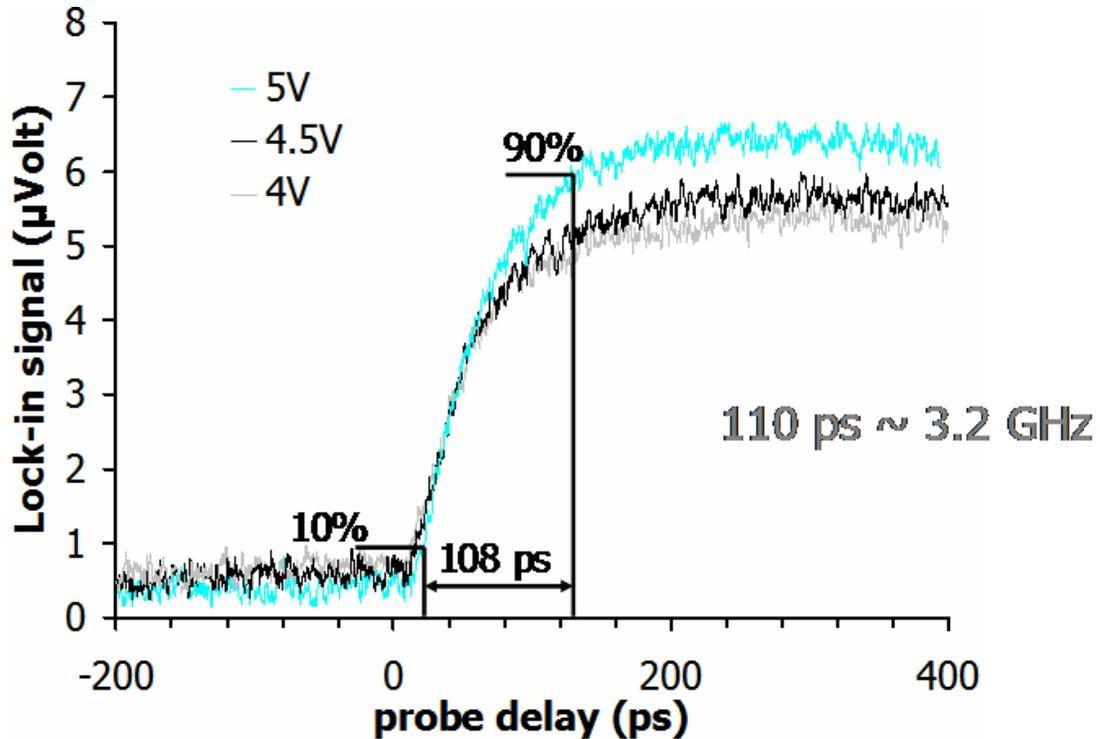
Figure 5.7 Pump-probe measurements of the rise time of a 6  $\mu\text{m}$  finger spacing planar P-I-N SOI detector for 4, 4.5, and 5 V bias
