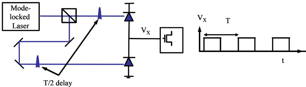
Figure 4.1 Receiver-less square wave clock generation at a high-impedance node ( $V_x$ ) using optically differential delayed mode-locked laser pulses
