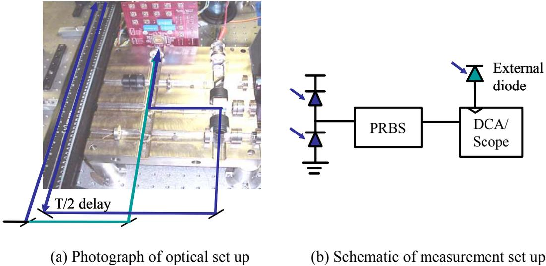
Figure 4.4 Photograph and schematic diagram of the experimental set-up
