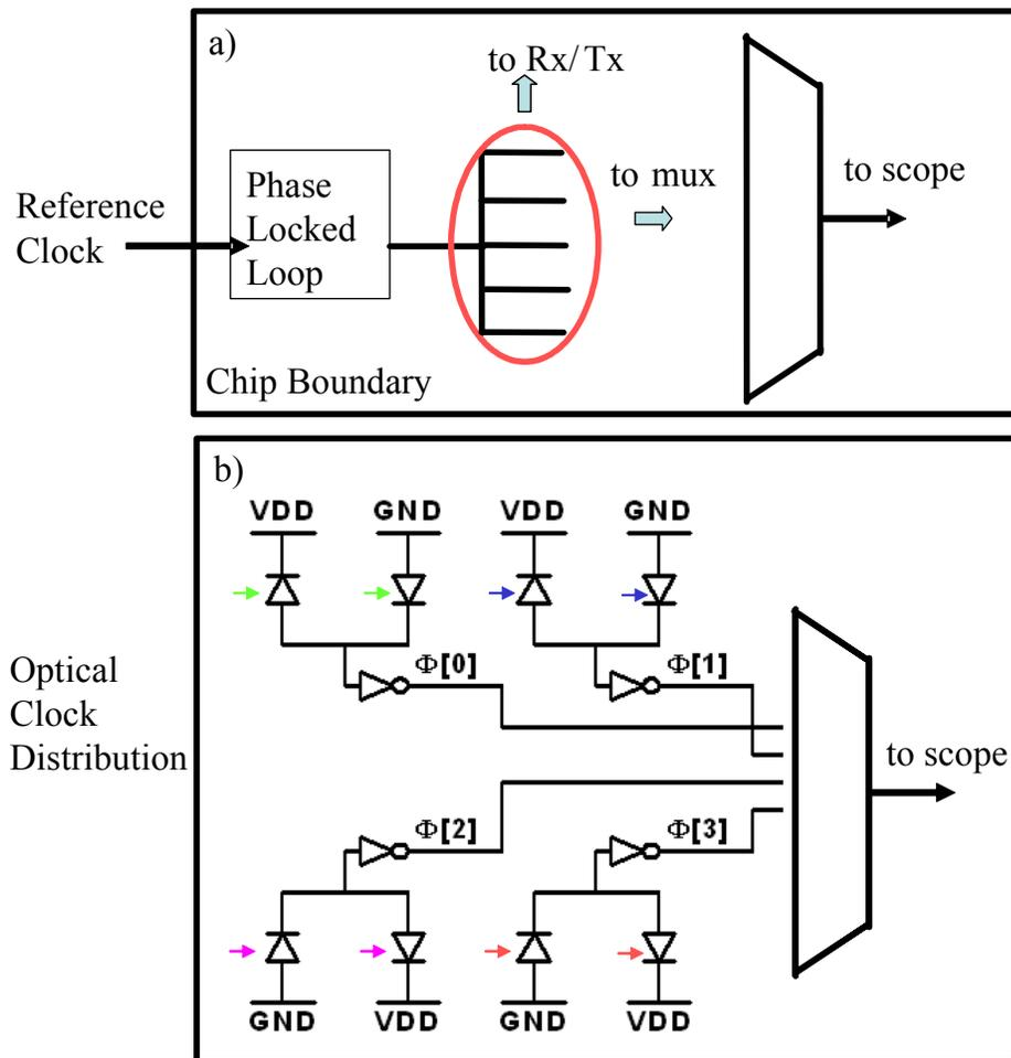
Figure 6.4 a) Electrical clock distribution for an optical link chip b) Optical clock distribution with receiver-less clocking. Different timing of the optical pulse pairs' arrival at the photodiodes leads to the controllable generation of the clocks with different phases,  $\phi[1]$  to  $\phi[4]$
