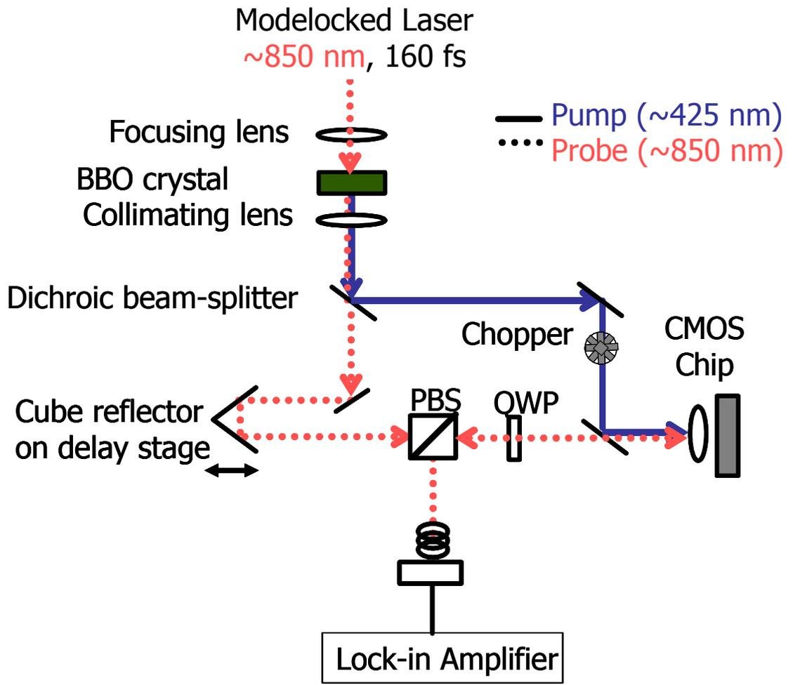
Figure 5.6 Experimental set up for pump-probe measurement
