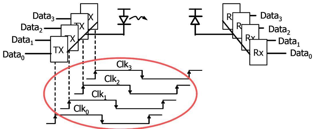
Figure 6.1 Optical link with four phase multiplexed clocking
