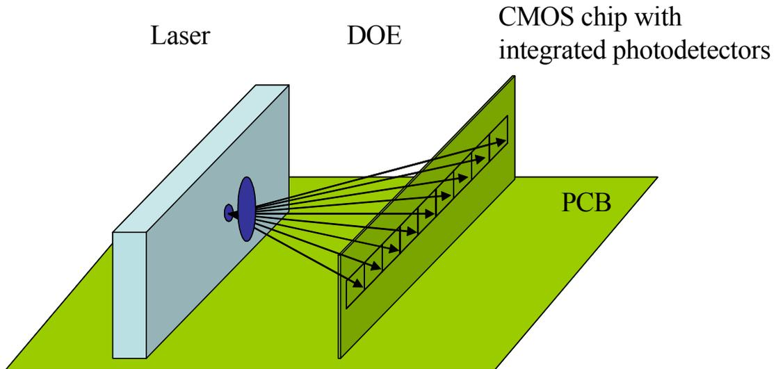
Figure 2.5 Free-space optical clock distribution uses a diffractive optical element (DOE) to generate an array of beams from a single laser and focus them onto individual photodetectors integrated on a CMOS chip
