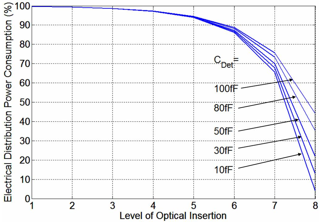
Figure 3.5 Electrical power consumption vs. level of optical injection for different photo-detector capacitances (1 GHz)
