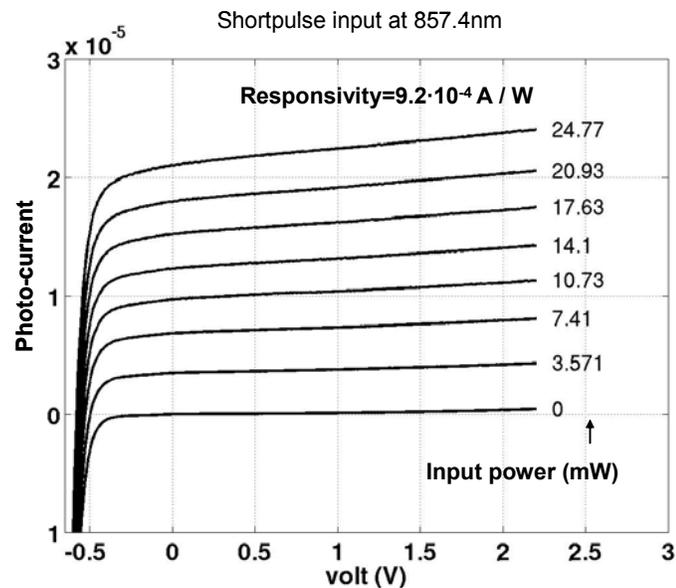
Figure 5.13 I-V curves for 2.4  $\mu\text{m}$  spacing SOI detector with  $\sim 425$  nm short pulse light
