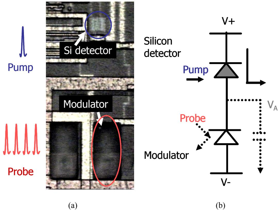
Figure 5.5 (a) Flip-chip bonded GaAs-AlGaAs MQW devices with SOI CMOS detectors. The probe delay is swept. (b) Schematic of detector-modulator connection
