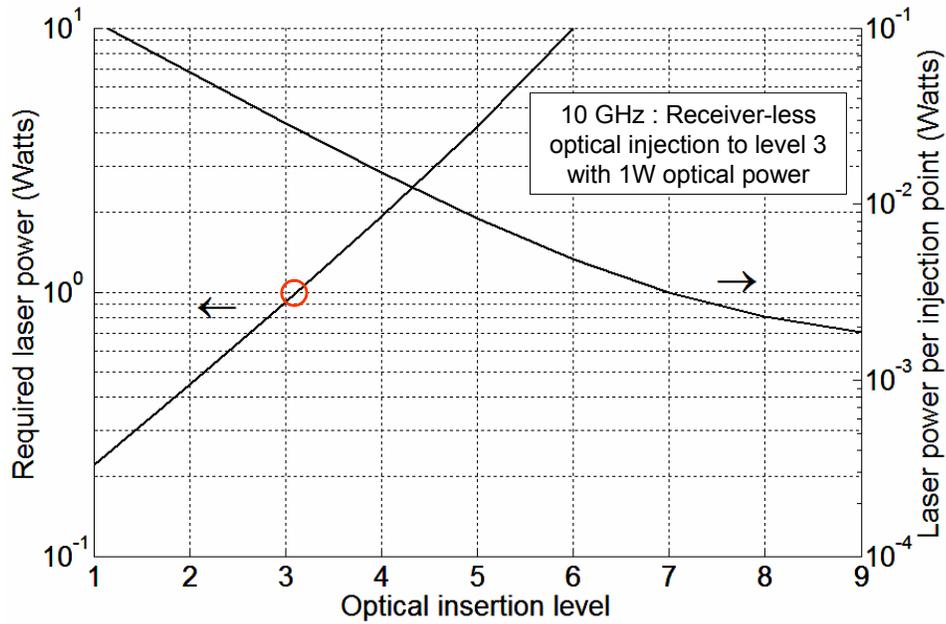
Figure 3.9 Laser output power required for optical clock injection vs. insertion level. (Right axis) Laser power required per injection point (10 GHz)
