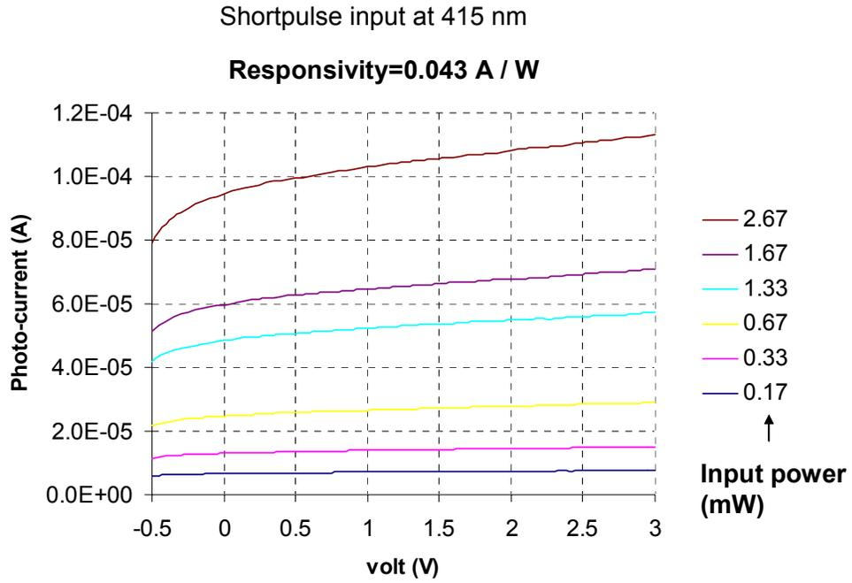
Figure 5.14 I-V curves for 6  $\mu\text{m}$  spacing SOI detector with  $\sim 425$  nm short pulse light
