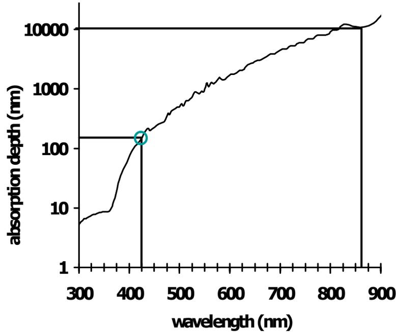
Figure 5.2 Absorption depth data for crystalline silicon vs. wavelength (adapted from S. Adachi [1])
