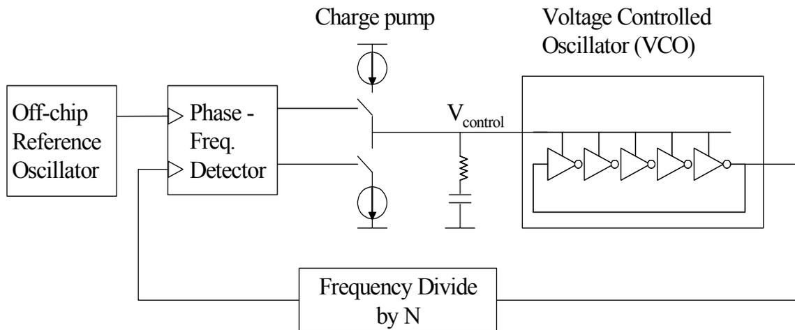
Figure 2.1 Block diagram of a Phase Locked Loop (PLL)
