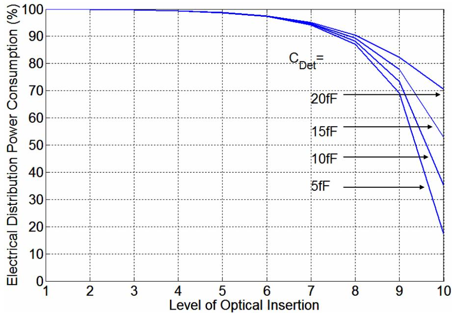
Figure 3.8 Electrical power consumption vs. level of optical injection for different photo-detector capacitances (10 GHz)
