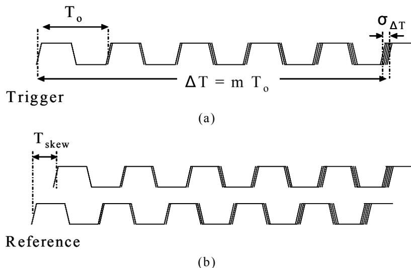
Figure 2.3 Pictorial definitions of (a) Jitter and (b) Skew
