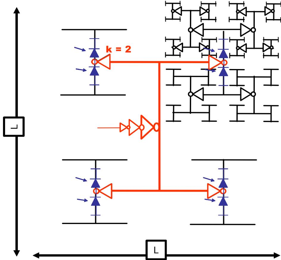
Figure 3.3 Optical clock injection to level  $k = 2$
