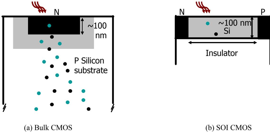
Figure 5.1 Responsivity-speed tradeoff in bulk and SOI CMOS photo-detectors for 850 nm light Depletion regions are shown in gray
