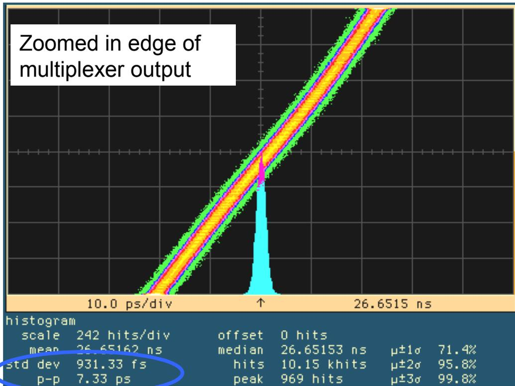
RMS jitter = 931 fs with optical clock
