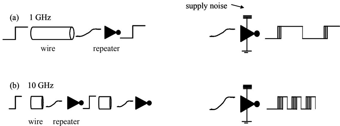
Figure 2.4 The effect of repeaters on wires at (a) 1 GHz and (b) 10 GHz
