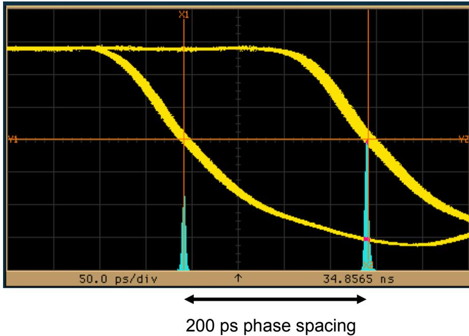
Figure 6.6 Overlay of two clock phases of the optical clock distribution showing a phase spacing of 200 ps, which was tunable over a 160 ps range
