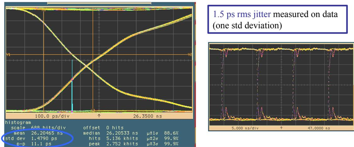
Figure 5.10 Zoomed-in picture of eye diagram of PRBS output when the PRBS is optically clocked using SOI CMOS photo-detectors and blue light. The histogram of the jitter on the falling edge is shown. A zoomed out version is also shown
