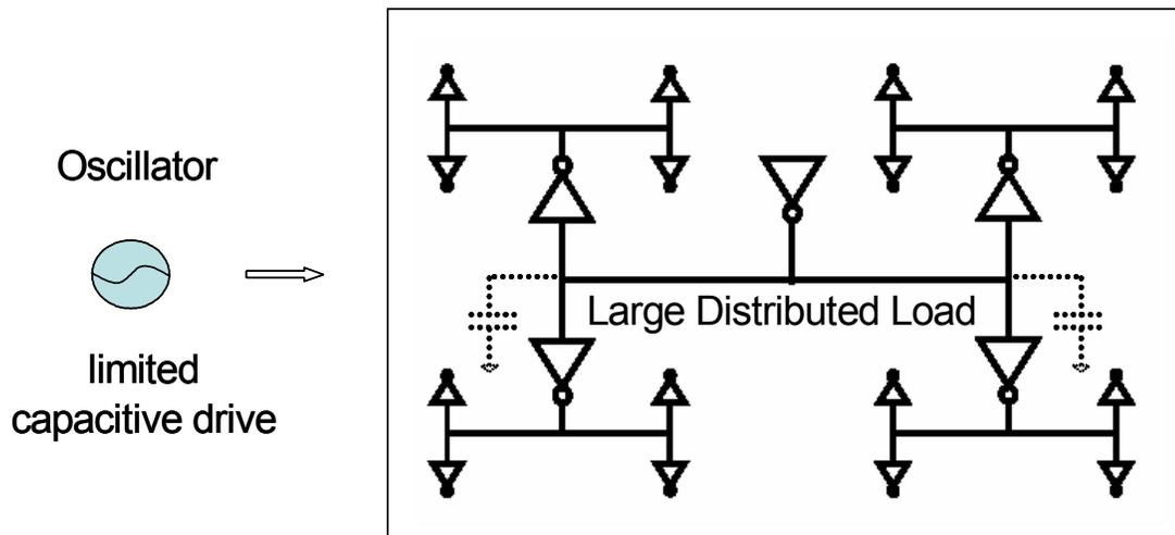
Figure 3.1 Electrical oscillator driving H-tree clock distribution with wires and repeaters
