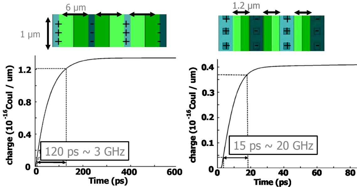
Figure 5.8 MEDICI simulations of the integrated photocurrent vs. time for planar p-i-n SOI detectors with 5 V bias for 6 μm and, in the inset, 1.2 μm finger spacing
