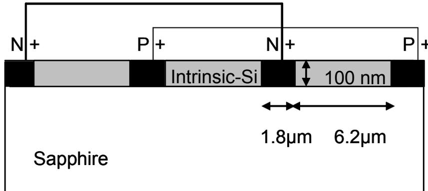
Figure 5.4 Schematic cross-section of a two finger lateral P-I-N SOI photo-detector
