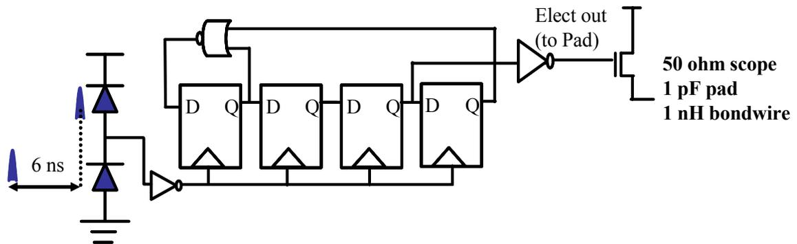
Figure 4.2 Pseudo-random-bit-sequence (PRBS) circuit with receiver-less optical clock. PRBS output viewed on scope after source follower, wire-bond and SMA cable
