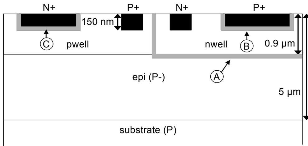
Figure 5.3 Schematic cross-section of photo-detectors in a bulk CMOS process. Junction areas are shown in gray and marked A, B, and C. Drawing is not to scale
