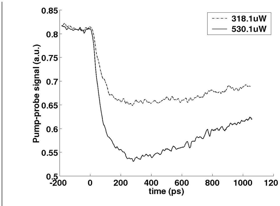
Figure 4.7 Pump-probe measurements of falling edge at the clock input to PRBS clocked by MQW detectors. Powers are per detector; 318  $\mu\text{W}$  and 530  $\mu\text{W}$  are shown
