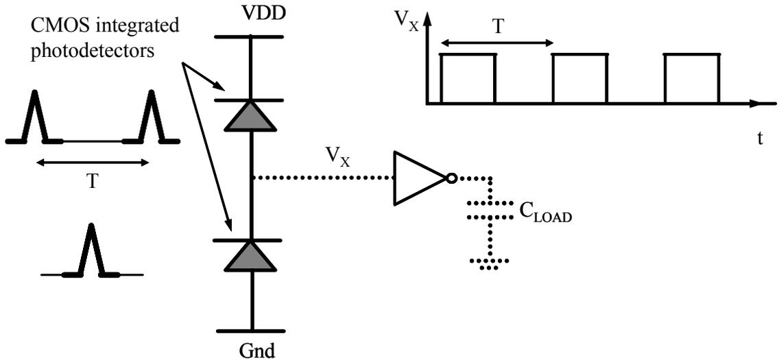
Figure 2.6 Full-swing optical clock injection using mode-locked laser pulses and receiver-less detection
