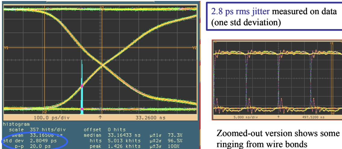
Figure 4.5 Zoomed-in picture of eye diagram of the output of the PRBS driven by the optical clock. The histogram of the jitter on the falling edge is shown. A zoomed out version is also shown
