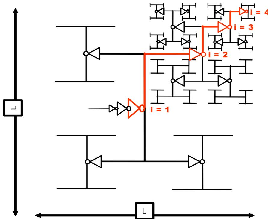
Figure 3.2 Geometrical H-tree model of electrical clock distribution
