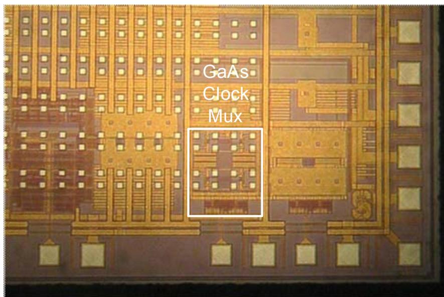
Figure 6.2 Optical clock-distribution for interconnects - test chip micrograph
