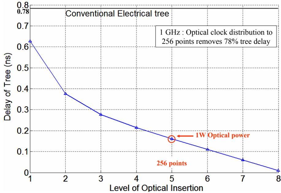
Figure 3.4 Total clock delay vs. level of optical clock injection for 1 GHz H-tree
