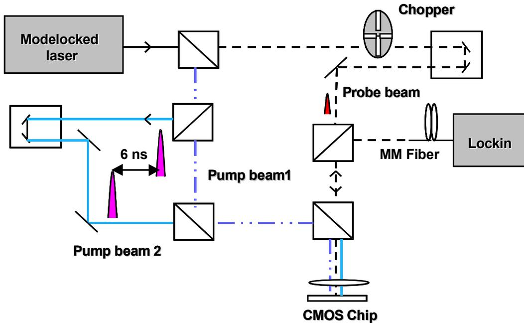
Figure 4.6 Schematic of three beam optical pump-probe set up to measure MQW detector transition time
