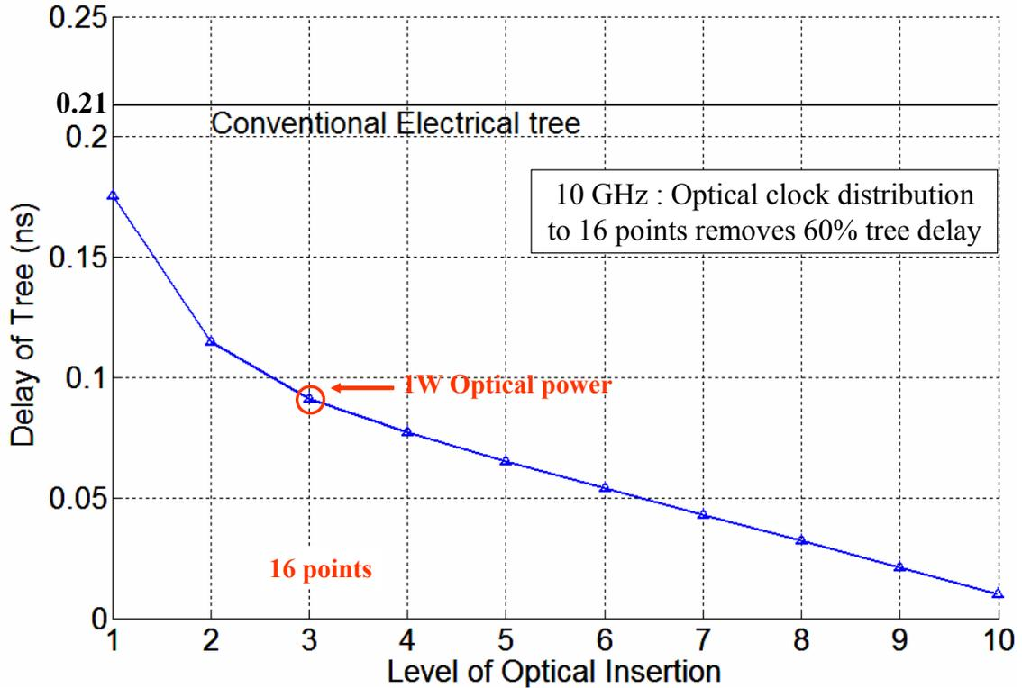
Figure 3.7 Total clock delay vs. level of optical clock injection for 10 GHz H-tree
