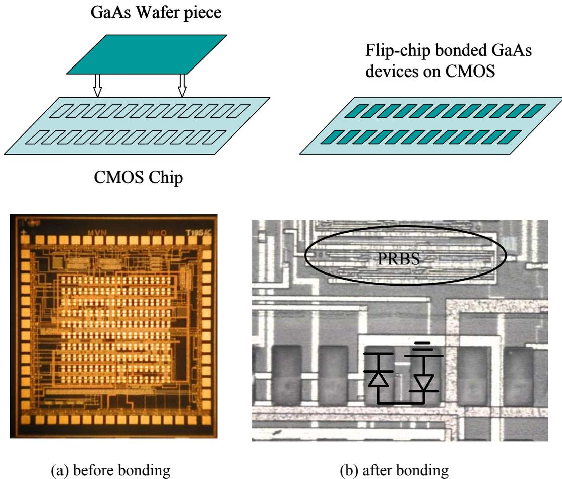
Figure 4.3 Conceptual diagram of the flip-chip bonding process (top row). Microscope photographs of the CMOS chip before and after bonding (bottom row). The PRBS and photo-detectors are marked on the zoomed-in photograph of the chip after bonding
