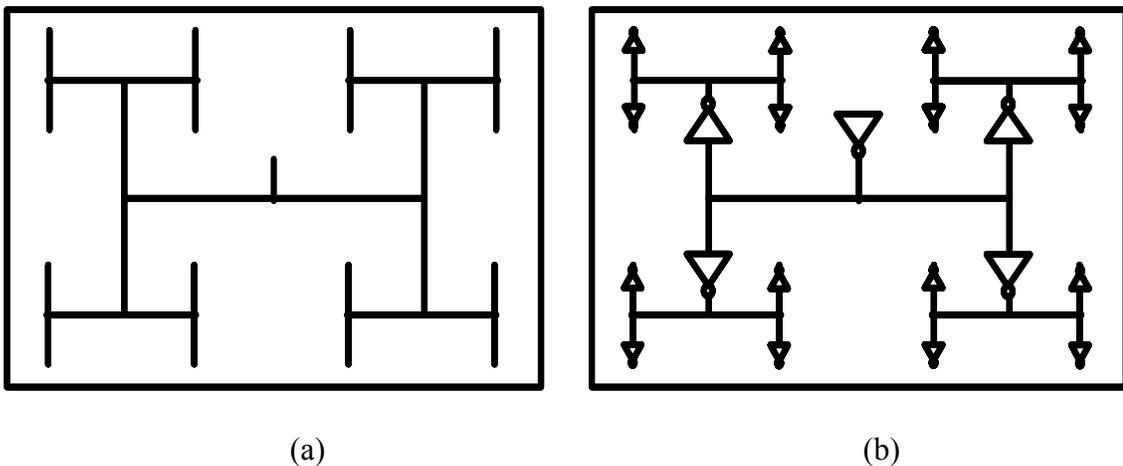
Figure 2.2 H-tree clock distribution with (a) wires only and (b) wires and repeaters
