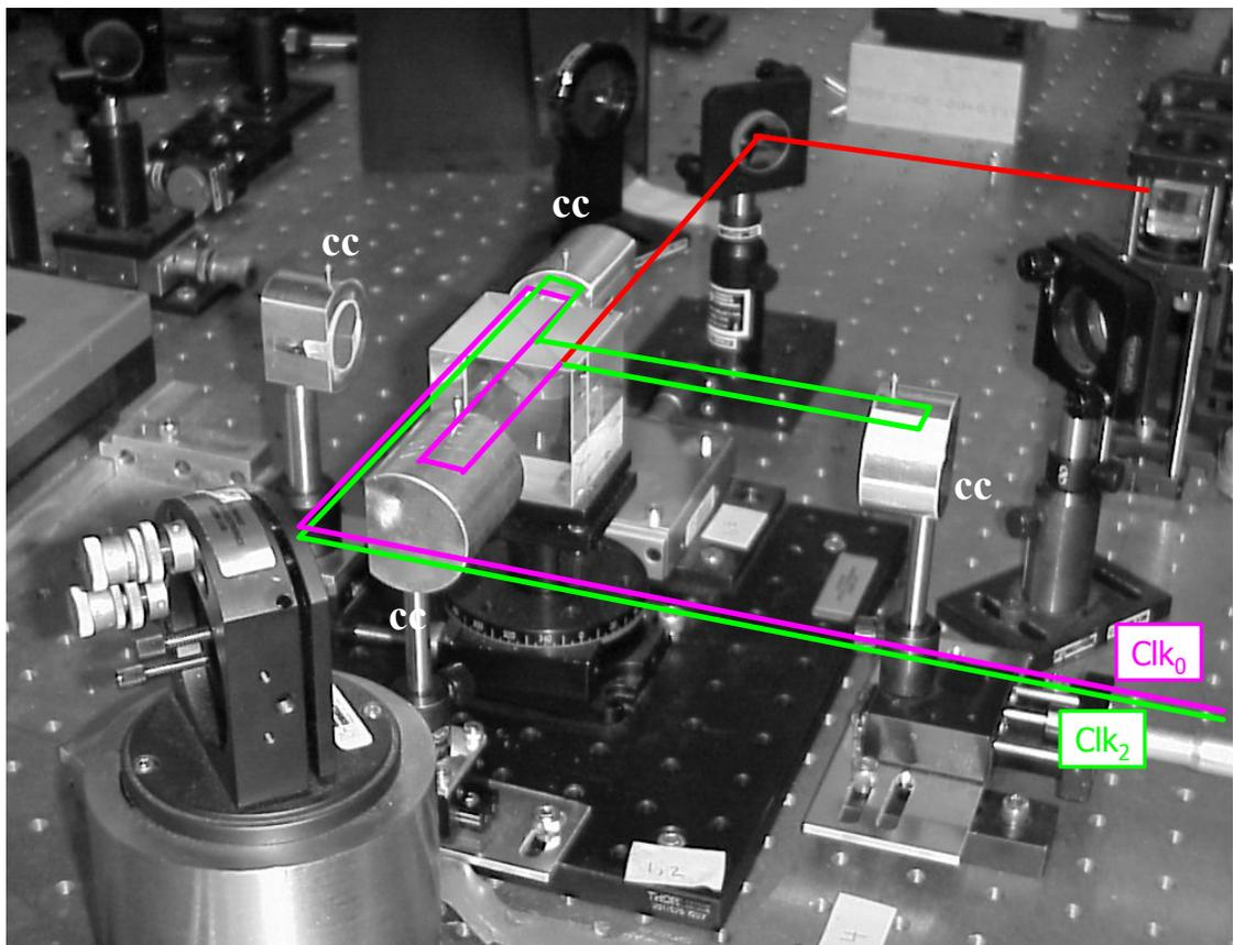
Figure 6.3 Optical setup for 4-phase clock spacing and distribution. Two beams shown for simplicity. The four corner cube (CC) reflectors are marked
