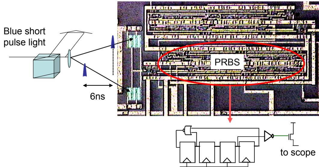
Figure 5.9 Experiment for optical clock injection to digital PRBS using blue light and SOI CMOS photo-detectors
